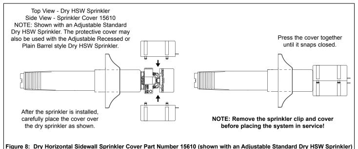
(Optional for temporary use with Viking Dry HSW Sprinklers until finish work is completed around the sprinkler.)
